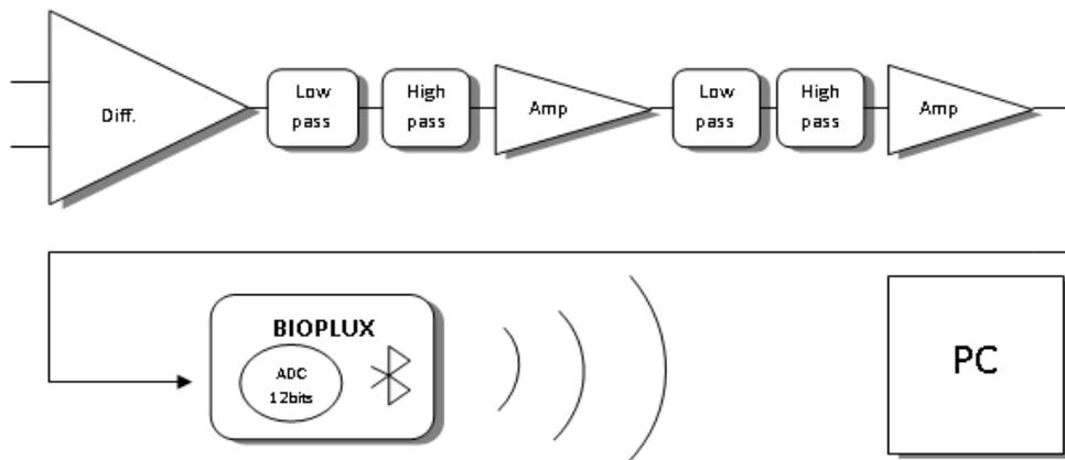
Fig. 1 - Diagram illustrating the acquisition and conditioning electronics.
