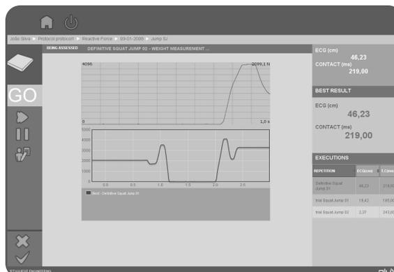
Figure 3: Evaluation screen showing the results of a counter movement jump evaluation.
